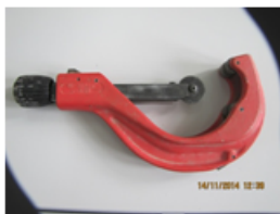
Fig. 2. Pipe cutter for different size pipes
