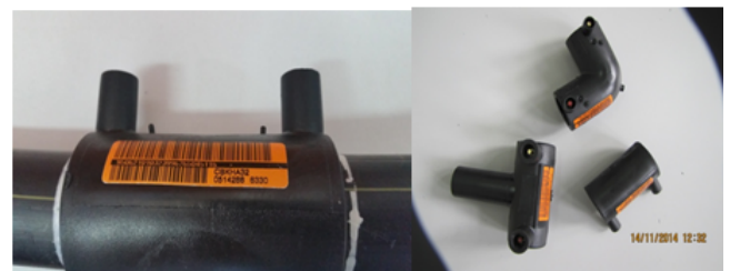
Fig.1. Threaded assembly consisting of 32 D diameter polyethylene fitting and Dn 32 PE 100 pipe; and polyethylenene fittings
